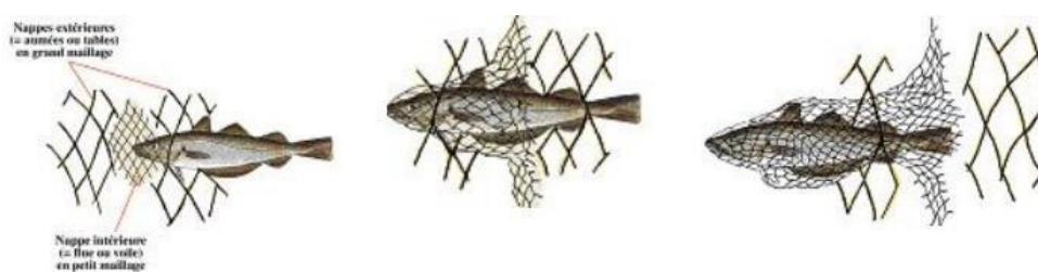
FIGURE 2 : CAPTURE AU FILET TREMAIL (SOURCE : IFREMER)
